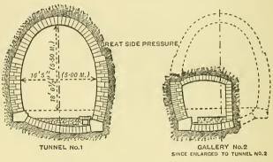
FIG. 4.-SECTIONS OF TUNNEL NO. 1 AND GALLERY NO. 2.
